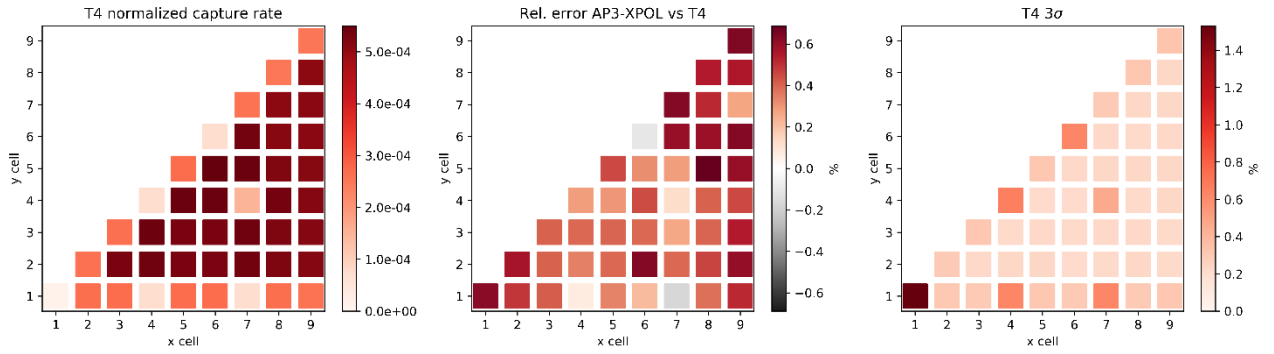
Figure B.8: Layer 8 comparison with TRIPOLI-4 ® for the capture rate
